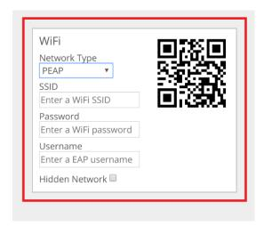
9. Turn on the headset, in the headset select scanner in the bottom row and then scan the QR code (Tip – hide or zoom in on the wifi so the proxy and enrol device QR codes are not showing on the screen) You will typically here a beep, the wifi symbol at the bottom of the screen should change to white
